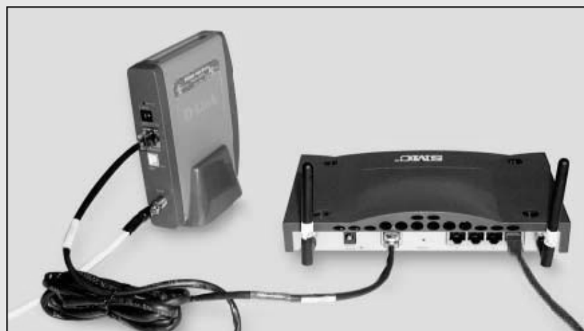
(Left: Cable Modem Right: Wireless router with LAN Ports- Ethernet Cables)
